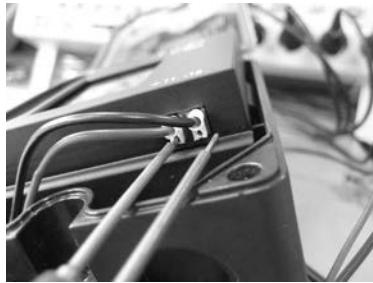
Fig. 14 · Cage clamp terminal with test contact
