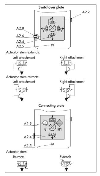
**Fig. 15:** Switchover plate and connecting plate on *Type 3277-5*
