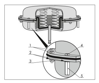
**Fig. 22:** Preloaded springs (functional diagram)
