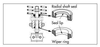
Fig. 19: Aligning the radial shaft seal and wiper ring
