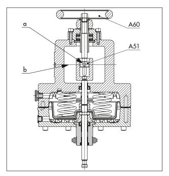
Fig. 17: Type 3271-5 Actuator with handwheel
