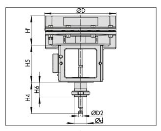
**Fig. 9:** *Type 3277-5* ⋅ 120 cm<sup>2</sup> actuator area
