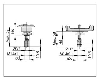
**Fig. 11:** Type 3271-5 and Type 3277-5 with 7.5 mm travel for Type 3510 Micro-flow Valve
