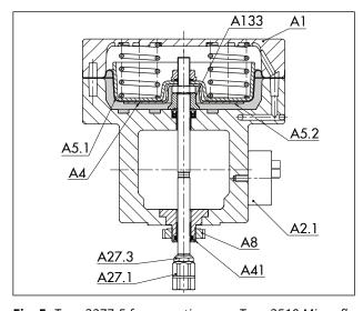
**Fig. 5:** Type 3277-5 for mounting on a Type 3510 Micro-flow Valve
