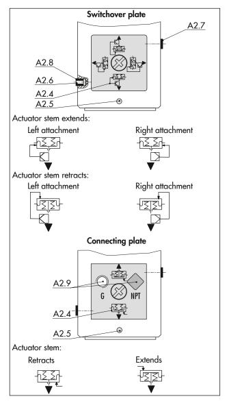
Fig. 6: Switchover plate and connecting plate on Type 3277-5
