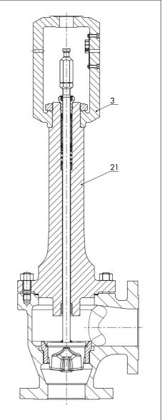
Fig. 9-2: Type 3256 with insulating section
