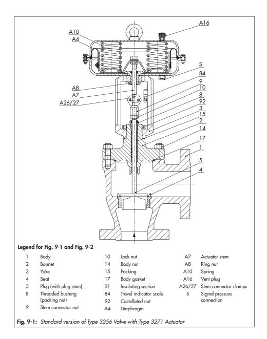
(22) onto the valve body, making sure that the hole of the plug that releases the flow first faces toward the valve outlet
