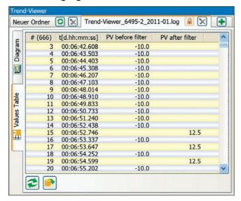
The values table contains all the measured data together with a time stamp of the parameters used in the Trend-Viewer.
