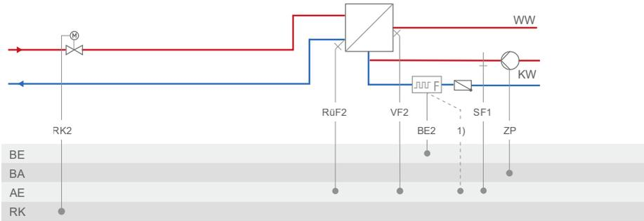
1) Terminal 11 when a vortex flow sensor is used
