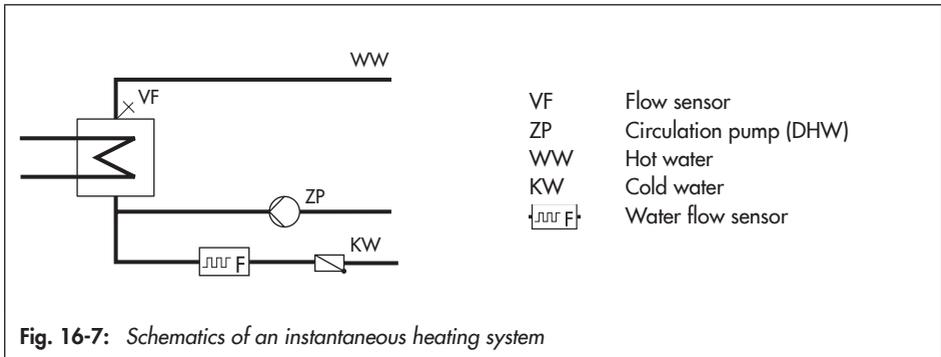
Fig. 16-7: Schematics of an instantaneous heating system
