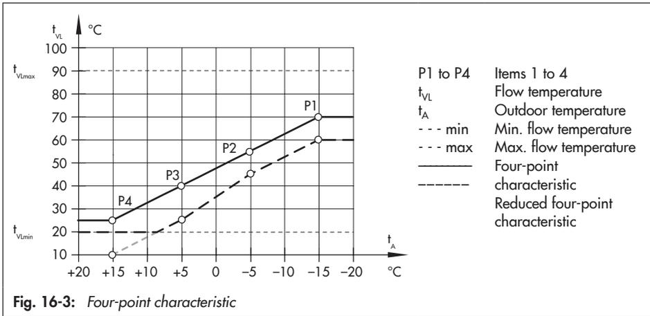
Fig. 16-3: Four-point characteristic
