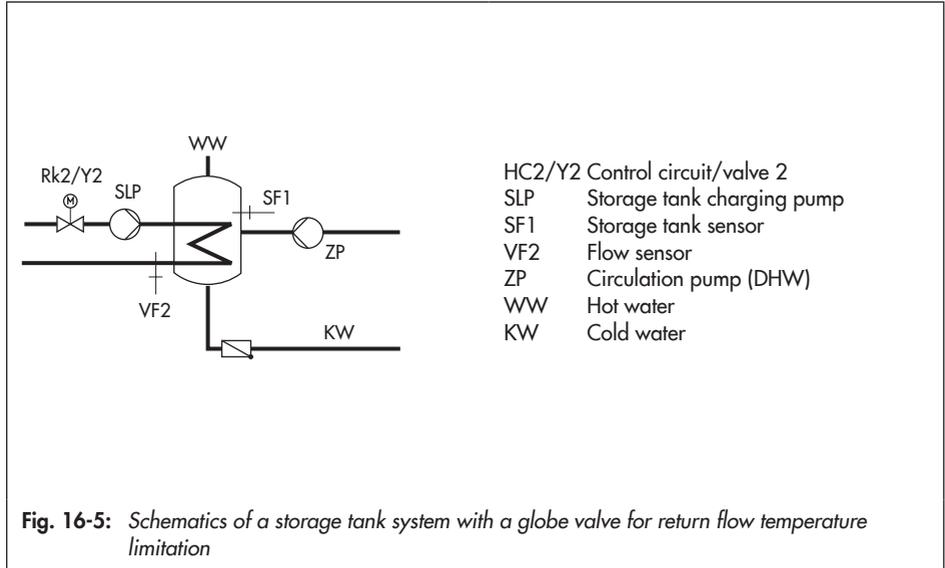
Globe valve and flow sensor VF2 are used exclusively for return flow temperature limitation in the schematics shown above. The pre-control circuit provides at least the same flow temperature as in the standard schematic version which is calculated from 'DHW temperature set point' + 'Charging temperature boost' + 'Boost set point (pre-control circuit)'.
