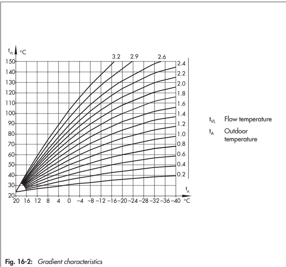
Fig. 16-2: Gradient characteristics
