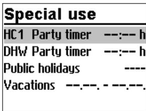
Turn the rotary switch to **#** (special times-of-use). The party timer for the first control circuit is now selected.
