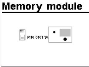
During data transfer, the zeros and ones run across the display. When the transfer was successful, 'OK' is displayed. After that, the connection between controller and memory module/mini module can be terminated.
