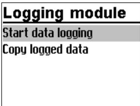
The data logging module is plugged into the RJ-45 connector socket located at the side of the controller. Once the module has been connected, 'Start data logging' and 'Copy logging data' appear on the controller display.
